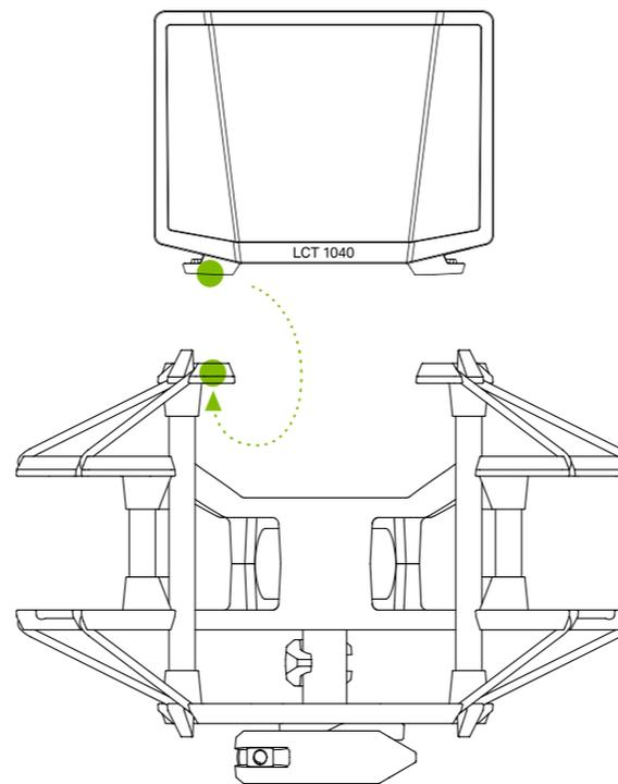
Mount the shock mount onto a stable microphone stand. Open the fixture of the shock mount. Put the tube microphone in the shock mount. The tube window indicates the default front. Lock the fixture.
