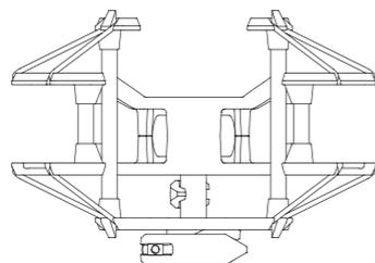
Shock mount that reduces low-frequency rumble and structure-borne noise
